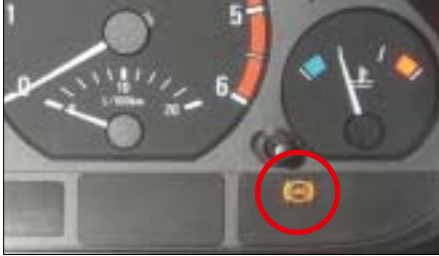
The ABS warning lamp is lit.
